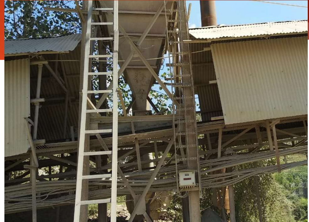
Fig.-1.10 Dust Collector attached to Crusher
