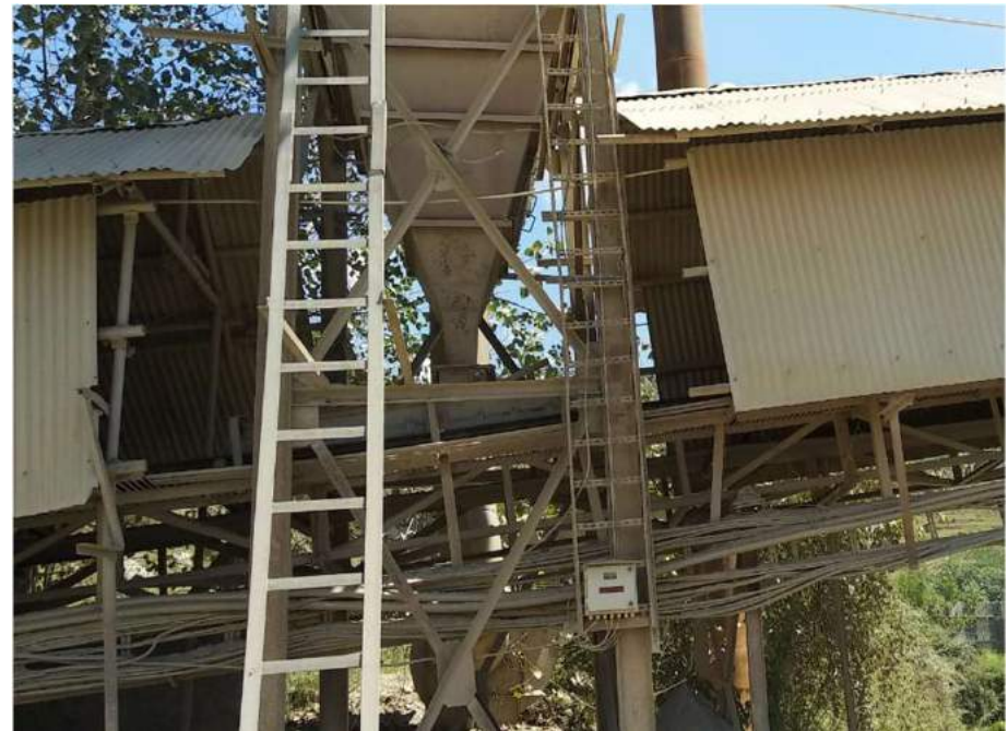
Fig.-1.10 Dust Collector attached to Crusher
